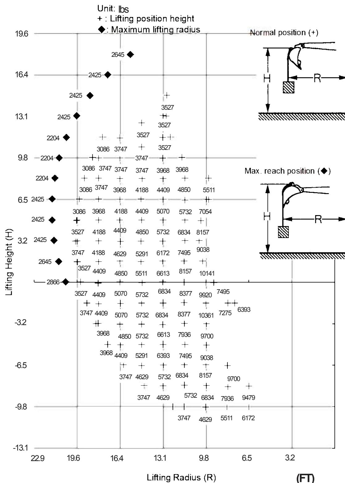
Boom cylinder lifting capacity (SAE method)
